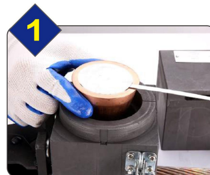
Insert ESTWELD® SAFE package into mold
