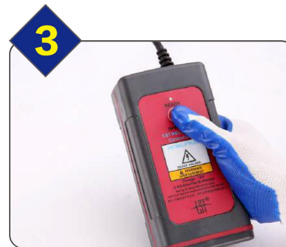
Press and hold control unit switch and wait for the ignition
