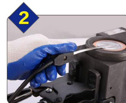
Attach control unit termination clip to igniter strip
