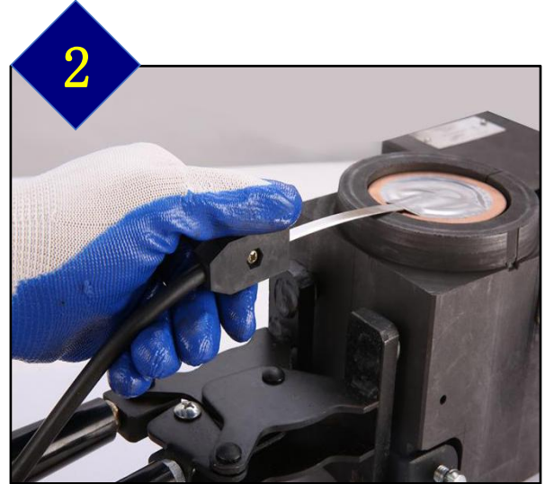
Attach control unit termination clip to ignition strip.
